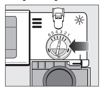
The dosage adjuster in the opening has settings from 1 to 6 (1-6 ml). It is set to 3 (3 ml) at the factory as the recommended dosage for **rinsing agent**.
