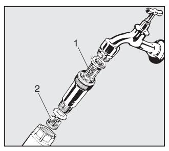
■ Clean the large area filter (1) and fine filter (2), and replace with new filters if necessary.
