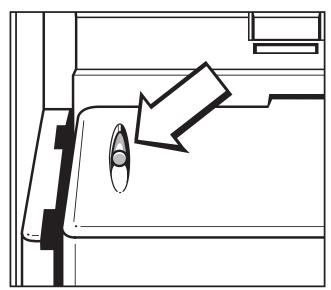
Press the reset button on the heater limiter (yellow) located on the lefthand side of the plastic cover.
