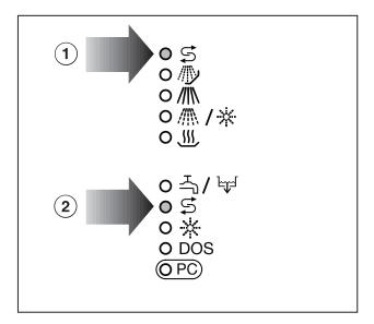
When the salt reservoir is empty the \$\mathref{5}\$ indicator light 2 comes on to remind you to fill the reservoir.
