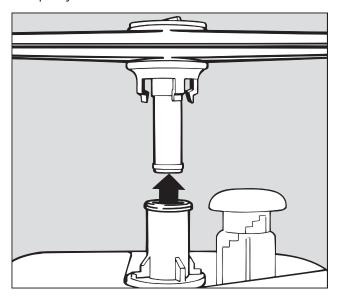
■ First remove the bottom basket and then pull the **lower** spray arm off.
